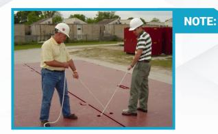
Barges can be pulled together by utilizing rope and the rope thimbles (tube turns) located along the perimeter of the deck.
