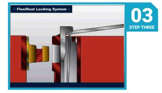
Turn pry bar over and push it through the opening in the upper locking bar casting.
