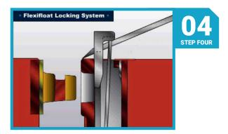
Lift pry bar and continue raising locking bar until the opening in the female lock casting is completely clear and the locking bar stops.
