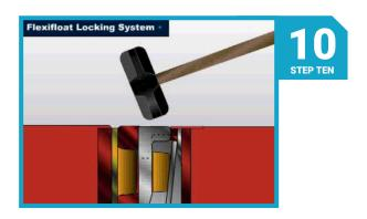
Drive locking bar until the spring bar secures in place under the two protrusions at the back of the female lock.
