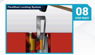
Begin driving the locking bar starting at the first connector location on one end of the row.
