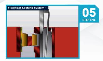
Repeat Steps 1 through 4 for all connectors along the row. Be sure all locking bars are completely raised; otherwise the connection cannot be completed.
