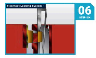
Drift the Flexifloats together, using hand lines until the male pin enters the female lock casting.
