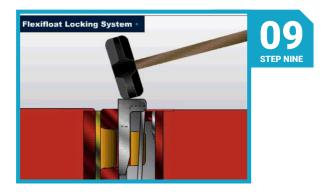
Continue driving the locking bar. If driving becomes difficult or a "metal-on-metal" sound is heard; stop, raise the locking bar, and reinspect the vertical gap to ensure both the top and bottom male pins are being engaged, then continue driving.
