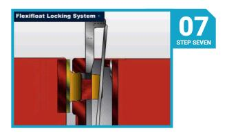
Continue to pull the adjoining Flexifloat rows together until the shoulder of the male pin is in close proximity to the female lock casting. All upper and lower lock connections along the entire row must be in this position before attempting further lock operations.
