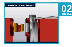
Insert pry bar into female lock behind the spring bar and raise locking bar upwards.
