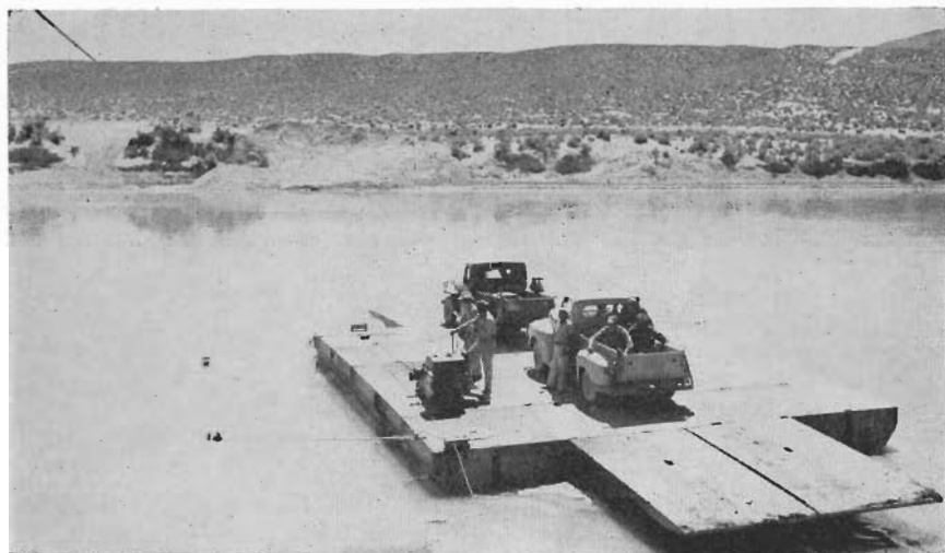
The five pontoon units and two ramp sections make a 65-foot long ferry which readily carries a truck and trailer or, as here, two vehicles.
