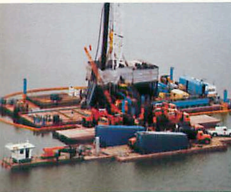
Top: Drilling operations under way in Lake Texoma. The two Flexifloat drive-on transport barges carry service trucks and drilling materials directly to the well site, thereby eliminating the need to rehandle material at the shore.
